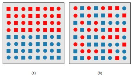
Fig. 4: An example of a boundary detection from Treisman's experiments: (a) a boundary defined by a unique feature hue (red circles and red squares on the top, blue circles and blue squares on the bottom) is preattentively classified as horizontal; (b) a boundary defined by a conjunction of features (red circles and blue squares on the left, blue circles and red squares on the right) cannot be preattentively classified as vertical
